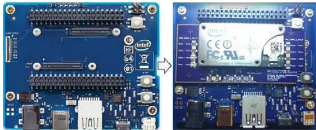
Figure 2: Left – expansion board with nothing plugged in; Right – compute module plugged into interposer, plugged into expansion board.
