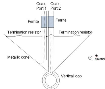
Figure 2: Proposed structure 2 of the resonance probe
