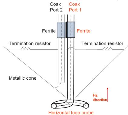
Figure 1: Proposed structure 1 of the resonance probe
