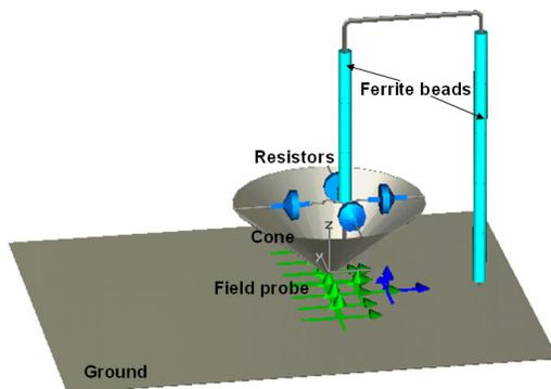
Figure 4: Cone structure above PEC in CST
