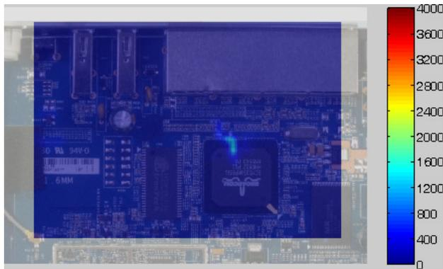
**Figure 11: Overlay of Susceptibility Scan and Injected Current Spread Scan shows USB Port related susceptibility areas and sensitivity levels (With External TVS - Figure 7b)**
