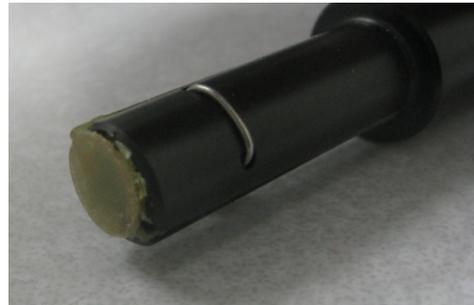
Figure 1: Loop Probe with 10mm diameter
