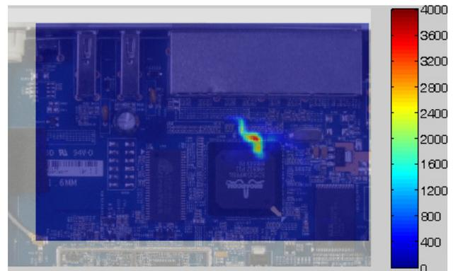
**Figure 10: Overlay of Susceptibility Scan and Injected Current Spread Scan shows USB Port related susceptibility areas and sensitivity levels (Without TVS – Figure 7a)**
