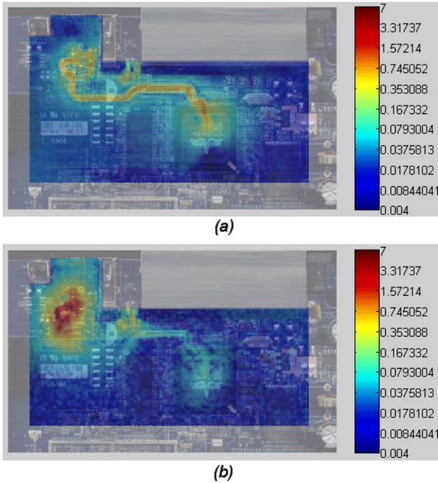
**Figure 7: Higher currents carried to integrated on-chip protection (a) than with discrete TVS (b)**
