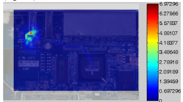
**Figure 9: Zoomed Current Spreading Scan via USB port injection**
