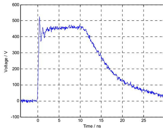
Figure 2: Injected modified TLP waveform into 50 ohm load
