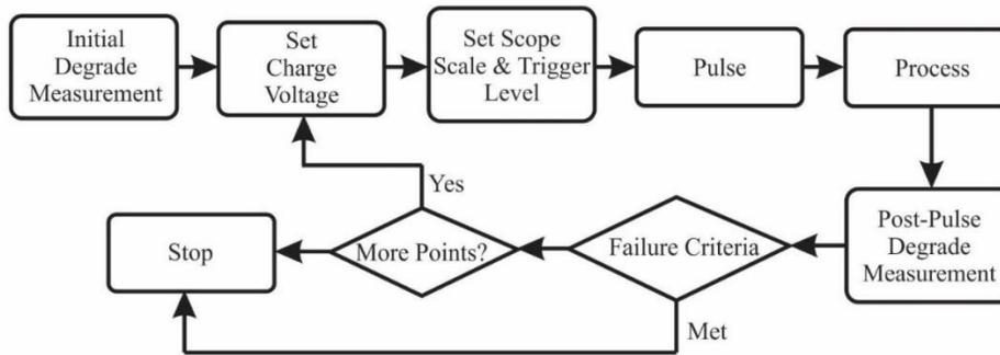
Fig. 4. ESDEMC TLP test procedure flow chart
