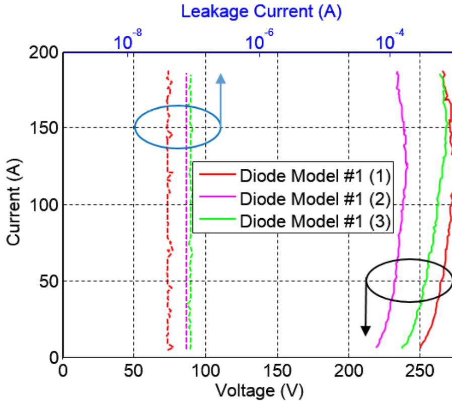
Fig. 7. Diode model #1 dynamic IV and leakage current curves.
