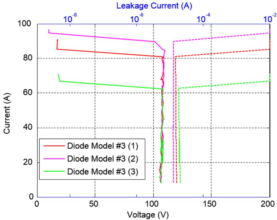
Fig. 11. Diode model #3 dynamic IV and leakage current curves.
