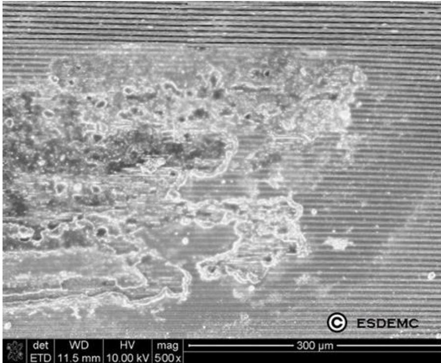
Fig. 2. SEM image of die surface from ESD damaged PV bypass diode sample, melted metal and silicon observed
