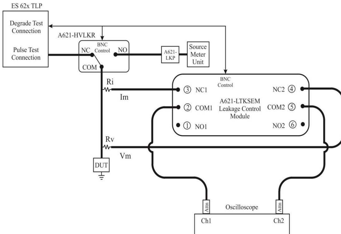
Fig. 3. ESDEMC High current TLP test setup for solar PV module diodes
