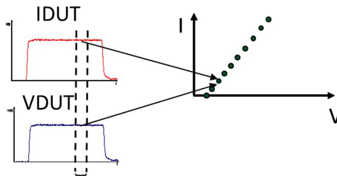
Fig. 5. TLP test dynamic IV curve obtain method
