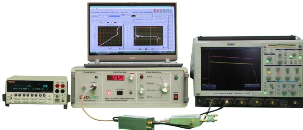
Fig. 6. PV Module TLP Test Configuration Photo
