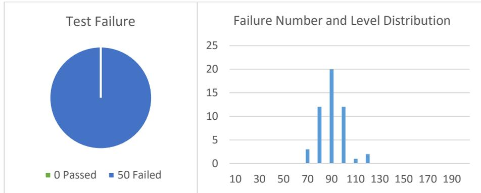
Fig. 12. Diode model #3 Failure Rate @ High Current TLP Test
