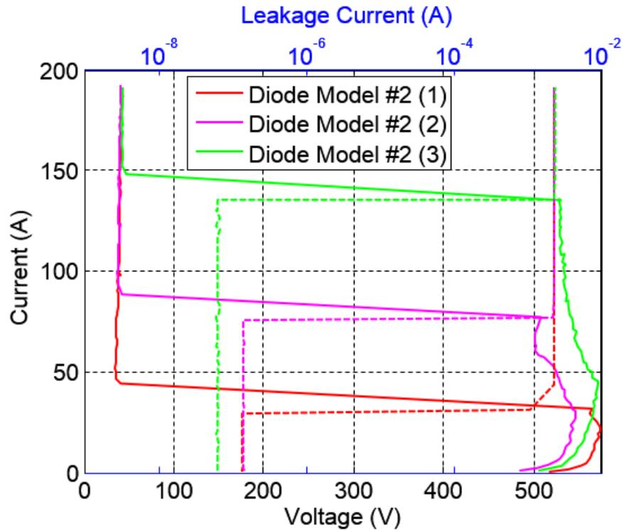
Fig. 9. Diode model #2 dynamic IV and leakage current curves.
