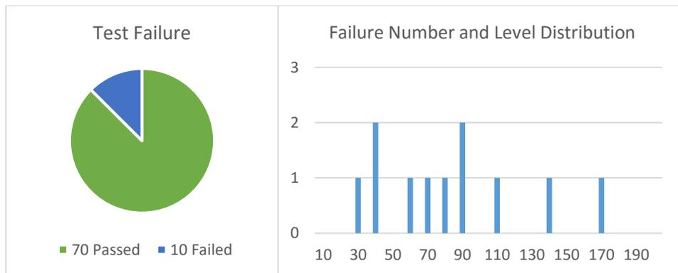
Fig. 10. Diode model #2 Failure Rate @ High Current TLP Test
