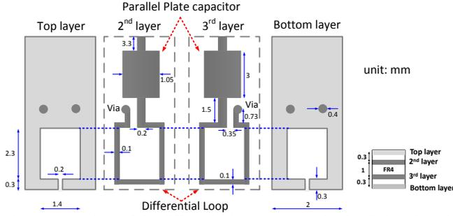
Fig. 1. Dimensions of the differential-loop resonator for the GPS probe. The differential loop is located at the tip of the resonator and then connected to the parallel-plate capacitor. The resonators of GSM and WiFi probes are similar.
