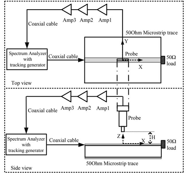
Fig. 4. Measurement setup for investigating the effect of cooling on the Q-factor, noise floor and sensitivity.
