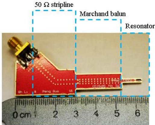
Fig. 3. Picture of the magnetic field GPS probe. The pictures of GSM and WiFi probes are similar.
