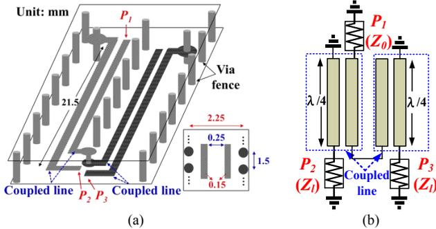
Fig. 2. (a) Dimensions and (b) equivalent circuit of the Marchand balun for the GPS probe. The baluns of GSM and WiFi probes are similar.
