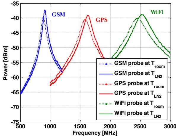
Fig. 5. Variation of the Q-factor for the GSM, GPS, and WiFi probes.  $T_{room}$  indicates room temperature.  $T_{LN2}$  indicates that the probe is cooled with liquid nitrogen.
